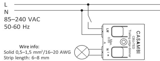
Never connect inductive loads, such as iron core transformers. This could cause permanent damage to the dimmer. Do not mix different types of loads.
