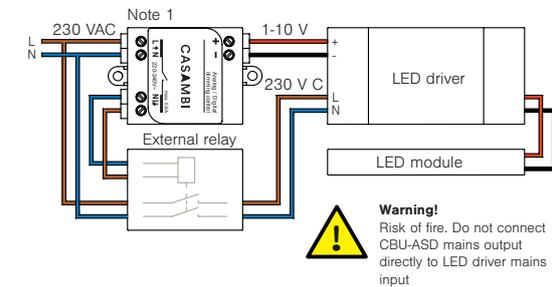
Note 1. CBU-ASD is a built-in class II device. Use double insulated wires or an external mounting box if the device is not mounted inside another insulated device.
