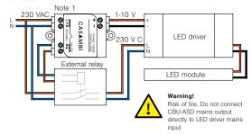
Note 1. CBU-ASD is a built-in class II device. Use double insulated wires or an external mounting box if the device is not mounted inside another insulated device.
